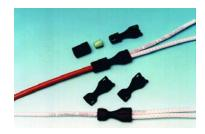
The Optical Fiber Duplexer enables cables with aramid strands to be broken out and mechanically terminated. It provides an easy-to-use assembly with no crimping, while still retaining a minimum of a 100N pull. Used with the 5mm diameter OFBLT at the output port, it gives full blend control and crush protection for ongoing fibers. The Duplexer gives an easy-to-use lay through facility with internal fiber radius control.
